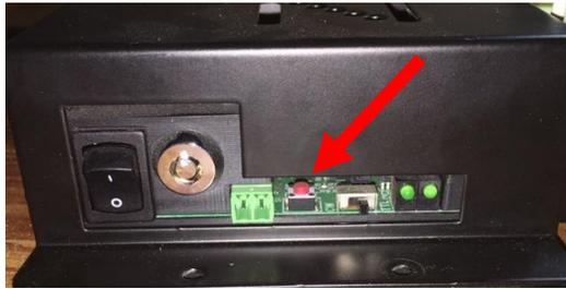
11.) Be sure the toggle switch is in TTL mode. TTL mode is used for controlling the Laser with your CNC and through Gcode. CW mode is for turning the laser on manually.
