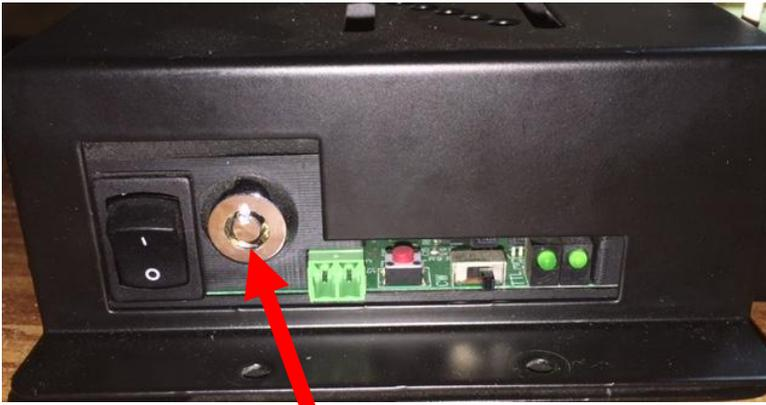
7.) Connect the **Signal Wire Connector** to your controller's signal wires (In This example we are using Pin 17). You will need to extend the harness as needed. Plug the other end (white connector) into the signal plug on the laser assembly.
