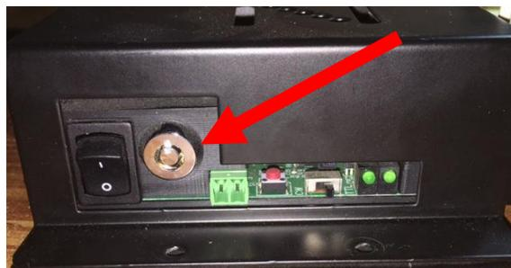
7.) Connect the **Signal Wire Connector** to your controller's signal wires. The Positive Signal Wire goes to the MS signal for the Z-Axis (originally the Z-Axis limit switch). The negative goes to the GND on the Z-Axis limit switch plug. You will need to extend the harness as needed. Plug the other end (white connector) into the signal plug on the laser assembly.
