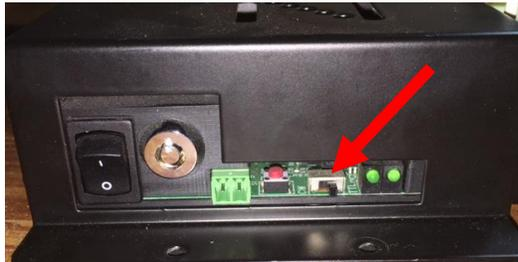
12.) With your glasses on, switch the main rocker switch to ON ("I"). Place a piece of scrap under the laser head and switch the laser to CW mode via the small toggle on the left side. The laser should illuminate. Go ahead and switch the toggle back to TTL to turn it off.
